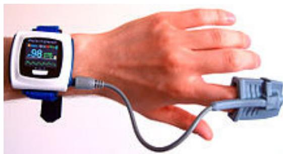
Figure 3. Mobile pulse oximeter.
