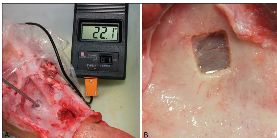
Fig. 2. Temperature measurement methodology. A , The thermocouple attached to the bone. B , The osteotomies accomplished by Er:YAG laser.
